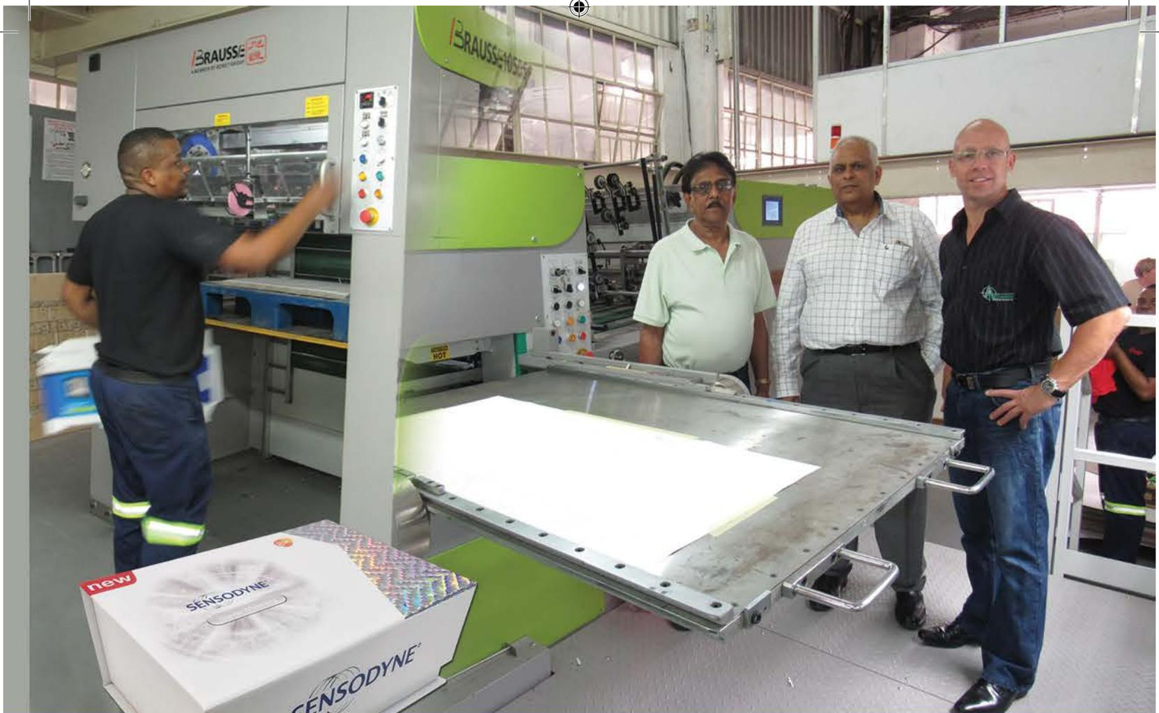
Above: Beneficial features of the die-cutting and stamping section include a pneumatic push button die-chase locking mechanism for safe and operator-friendly changing of the die; a double cam-driven gripper opener for smooth and accurate sheet register and take off; plus a 15mm insulation plate for optimising heating efficiency and maintaining a consistent temperature.
